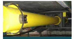
8" main-ram cylinder with up to 211,000 lbs. of platen force delivers up to 40% more force than competitive balers using 8" cylinders.
