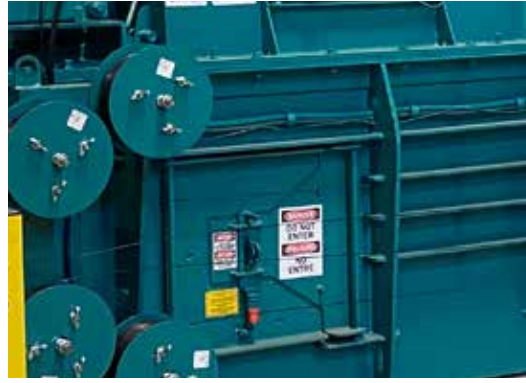
Lower ram chassis inspection door for easy maintenance access.
