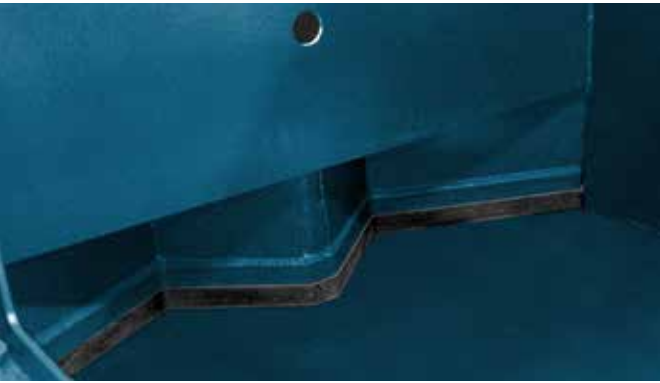
Hardened tool steel progressive shear blade and 46" penetration all but eliminates shear jams.
