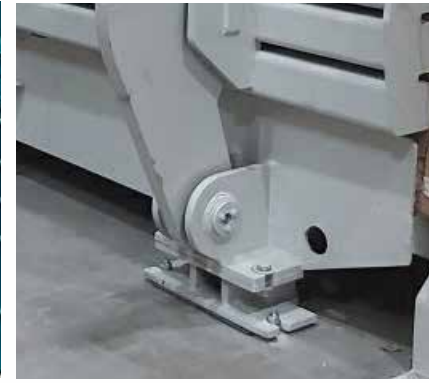
Raiser kit allows for easy cleaning and clearing around baler.
