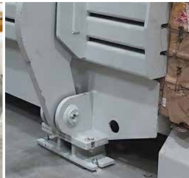
Raiser kit allows for easy cleaning and clearing around baler.
