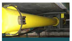
11" main-ram cylinder with up to 427,649 lbs. of platen force delivers up to 30% more force than competitive balers using 11" cylinders.
