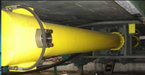
8" main-ram cylinder with 211,000 lbs of platen force delivers up to 40% more force than competitive balers using 6" cylinders.
