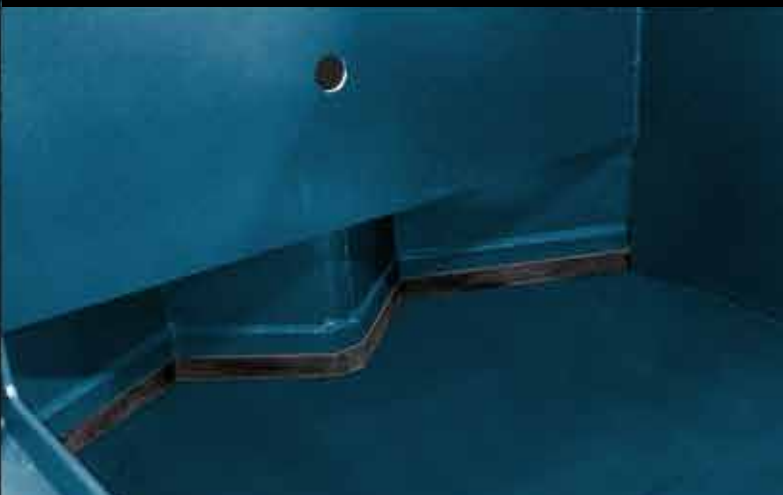
Hardened tool steel progressive shear blade and 30" penetration all but eliminates shear jams.
