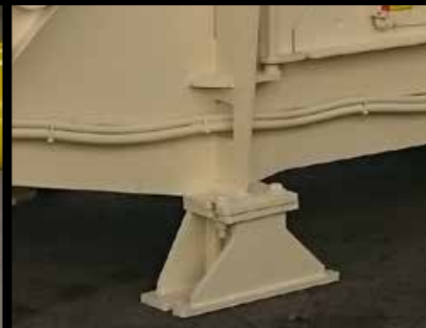
Raiser kit allows for easy cleaning and clearing around baler.
