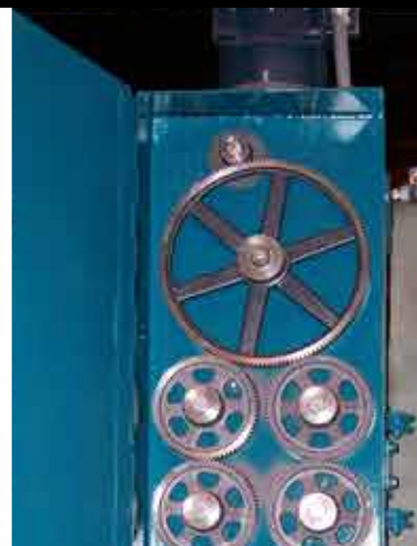
Maren's unique 100% gear driven twister maintains timing and avoids problems common with chain driven systems.
