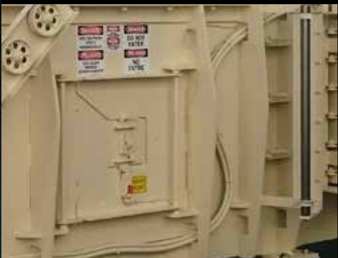
Lower ram chassis inspection door for easy maintenance access.
